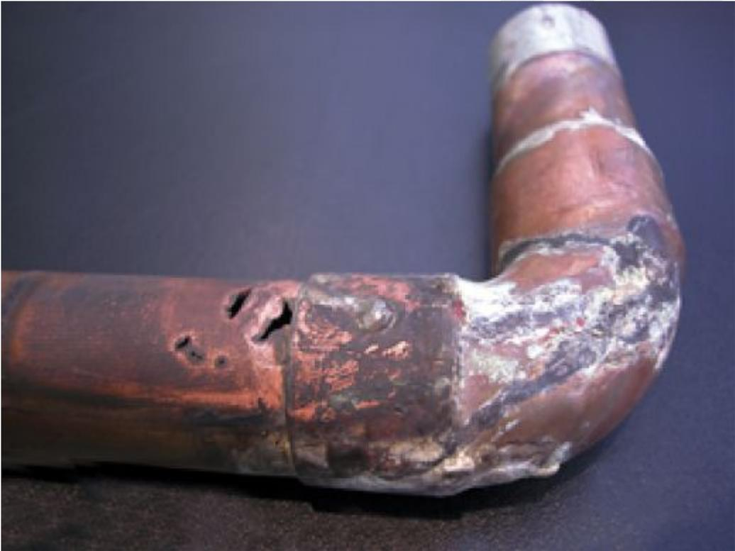
Figure 2. Pinhole leaks in copper tubing caused by internal corrosion.
