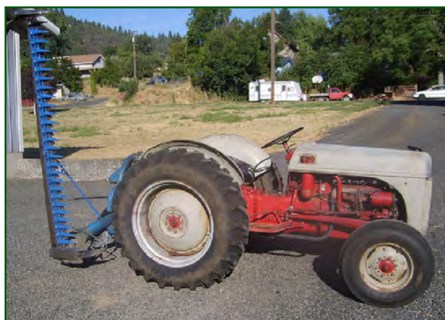
Figure 2. Sickle-bar type cutter. Photo by permission of Roger Kechter
