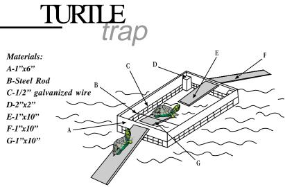
Figure 5: The trap need not be limited by these suggested materials or dimensions. Other similiar designs may be as effective.
