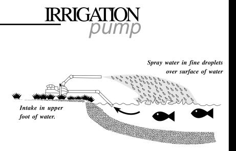
Figure 4 - Using an irrigation pump for aerating pond water.
