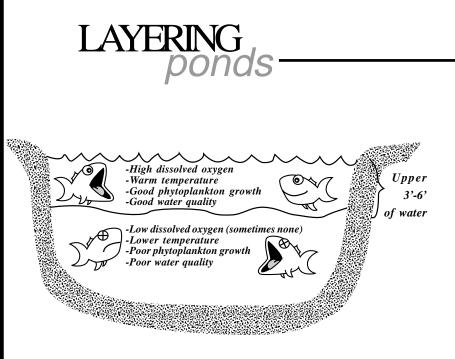
Figure 3 - Stratification (layering) of a fish pond in the summer.
