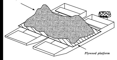
Figure 1 - A simple way of applying lime to a pond that is full of water.
